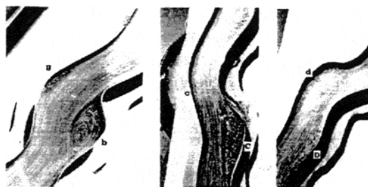
Fig. 4 Surface streakline in the model experiment
